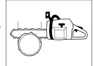
There are methods for felling trees with a diameter larger than the bar length. However these methods involve a much greater risk that the kickback zone of the bar will come into contact with the tree.
